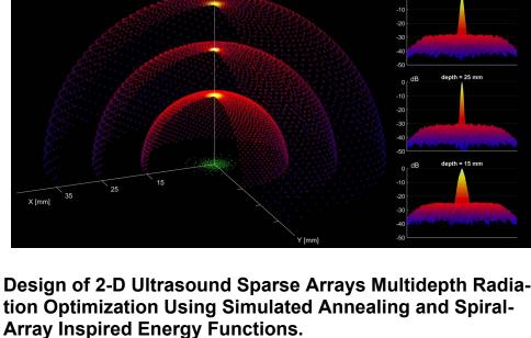
aimed at obtaining the same widths of the main and lower side lobe levels of the radiated pattern of a Blackman-tapered spiral ar-
